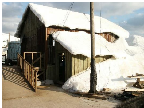
Snowy film decoration roofs by spraying PUR foam
